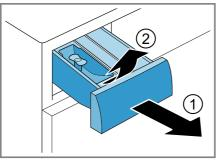
2. Remove the siphon cap by pulling it upwards, then clean the auxiliary compartment and siphon cap by rinsing with tap water or using a brush.
