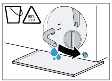
8. Firmly press on the sealing cap.
