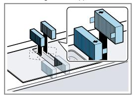
6. Insert the grease filter.
