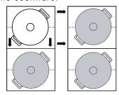
The cookware is detected and the previously selected power level and  ${\cal E}$  flash alternately on the display for the new cooking zone.
