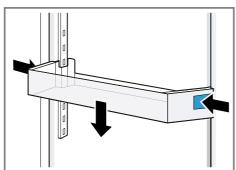
The height-adjustable door rack can be moved up without pressing the buttons.
