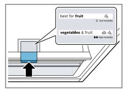
The air humidity in the fruit and vegetable container can be set according to the type and amount of food to be stored by pressing the humidity controller:
