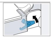
The hinge is now secured and cannot snap shut.
