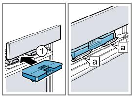
**9.** Slowly slide the control panel downwards and then push it away from you until it is closed completely.
