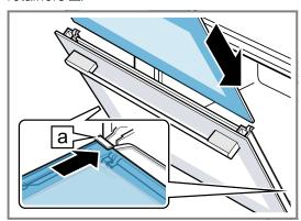
8. Push the inner pane upwards until it is in the left- and right-hand retainers a.
