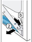
3. Tilt the condensate tray forwards slightly until the lower retaining hooks are released.
