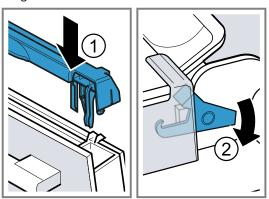
▼ The locking levers are closed. The appliance door is secured and cannot be detached. 12. Close the appliance door.
