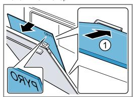
**5.** Push the inner pane in at the top ①. Push the sliding caps ⓐ downwards in the direction of the arrow.
