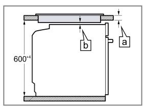
The minimum worktop thickness b a is based on the required minimum clearance a.
