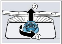
Pull down the micro filter to remove.
