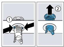
5. Clean the filter elements under running water. Carefully clean the rim of dirt between the coarse and the fine filter.
