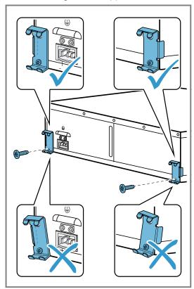
**6.** Slide the appliance into the fitted unit and check whether the tilt protection engages.
