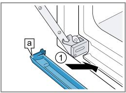
2. Snap the hooks a on the left and right of the condensate tray into the gap ①.
