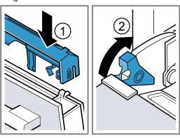
The locking levers are closed. The appliance door is secured and cannot be detached. 11. Close the appliance door.
