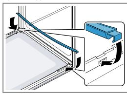
6. Slide the inner pane into the left- and right-hand retainers a.
