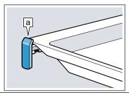
Note: The pull-out rails lock in place when they are fully pulled out. Gently push the pull-out rails back into the cooking compartment.
