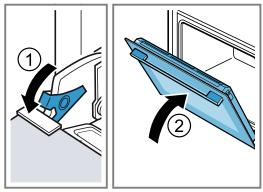
**4.** Push on the left- and right-hand side of the door cover from the outside ① until it is released.
