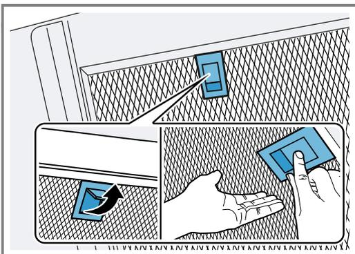
2. Remove the grease filters from the holders. To prevent grease from dripping, hold the grease filter horizontally.
