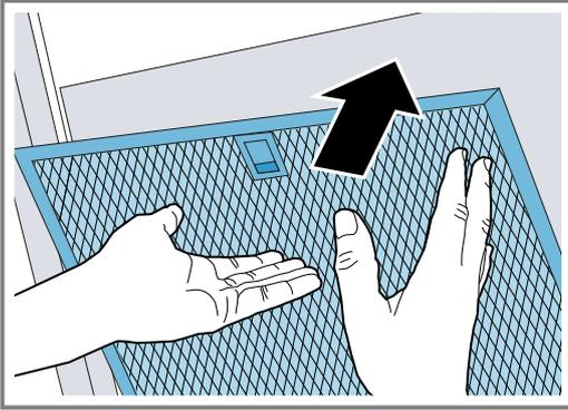
3. If the grease filter has been inserted incorrectly, carefully push the lock forwards, remove the grease filter and insert it correctly.
