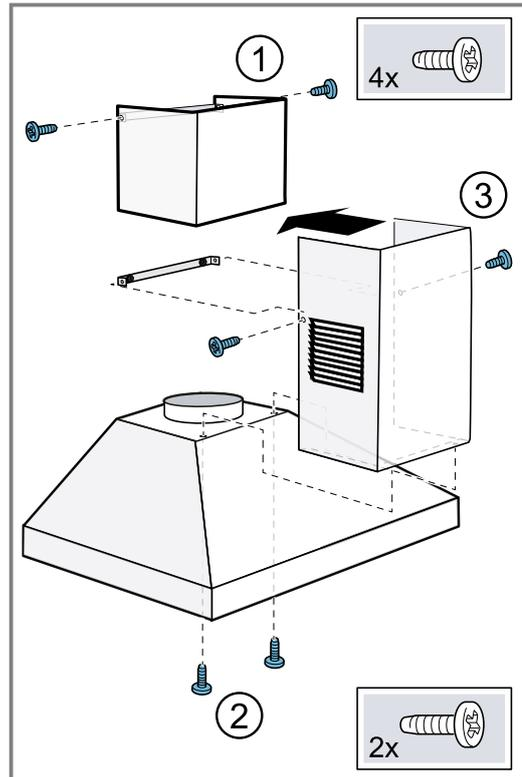
5. **Note:** To prevent scratches, lay soft towels over the edges of the outer flue duct to protect the surface. Place the lower flue duct on the appliance and pull it slightly apart.
