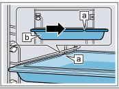
**3.** Push the accessory all the way in, making sure that it does not touch the appliance door.
