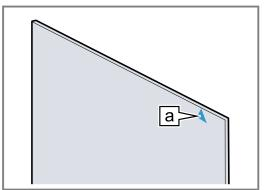
2. Insert the intermediate pane into the retainer a at the bottom ① and push it in firmly at the top.
