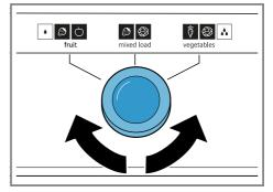
The air humidity in the fruit and vegetable container can be set according to the type and amount of food to be stored by turning the humidity controller:
