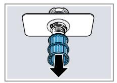
4. Press the locking catches 10 together and lift the coarse filter out
