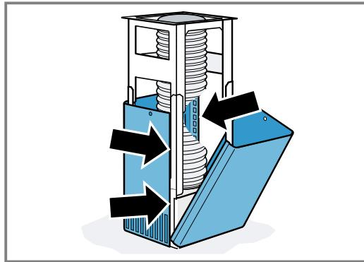
**Note:** The slots on the flue duct point downwards.
