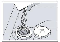
Fill the dispenser right up with special salt. The water in the dispenser is displaced and forced out.
