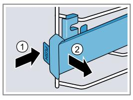
**3.** Pull the rail out towards the front until the retainer at the back unhooks.
