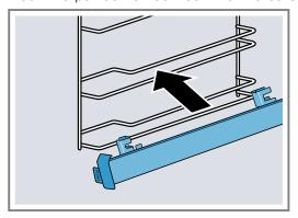
2. Push the retainer a in between the lower and the upper bar.
