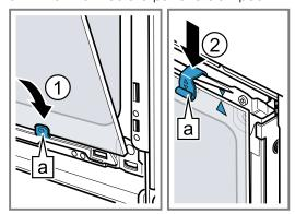
4. Attach the front pane downwards into the left- and right-hand retainers a 1.
