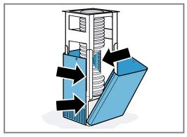
**Note:** The slots on the flue duct point downwards. Push the upper flue duct upwards and secure it using 2 screws.
