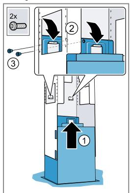
3. Hook in the retaining clips and screw them in tightly.
