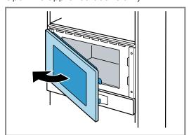
4. Screw the appliance to the unit on the opposite side to the hinges.
