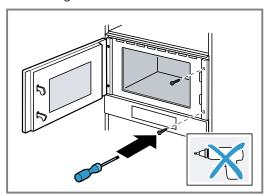
5. Pre-drill the screw holes in the unit on the side with the hinges.
