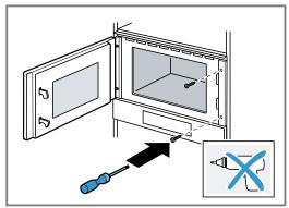
**5.** Pre-drill the screw holes in the unit on the side with the hinges.
