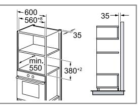
Do not fit the appliance too high up; it must be possible for accessories to be removed easily. Fit the feet.
