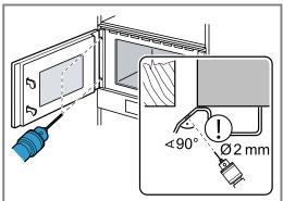
Cover the door hinges. Use a wood drill with a 2 mm diameter.
