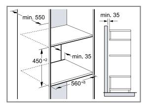
If the tall unit has another back panel in addition to the element back panels, this must be removed. Do not fit the appliance too high up; it must be possible for accessories to be removed easily.
