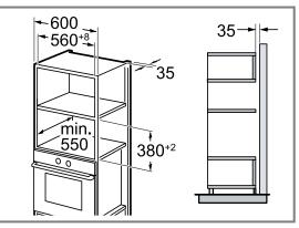
Do not fit the appliance too high up; it must be possible for accessories to be removed easily.
