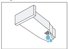
5. Remove the stopper on the underside.
