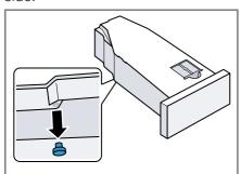
6. Insert the stopper into the recess in the top.
