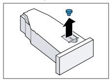
2. Insert the stopper on the underside.
