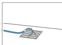
Secure the elbow to the gully.
