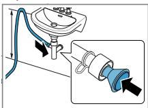
Secure the connection point with a (12-22 mm) hose clamp. Secure the water outlet hose with a hose guide at a height of at least 80 cm and no more than 100 cm.
