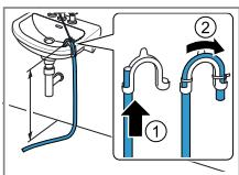
Push the water outlet hose fully through the elbow and secure it using fixing material. Secure the elbow at a height of no more than 100 cm.
