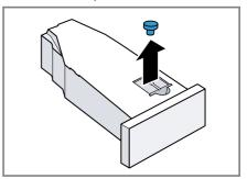
2. Insert the stopper on the underside.
