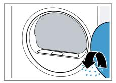
3. Remove the two-part fluff filter.
