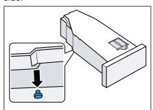
6. Insert the stopper into the recess in the top.
