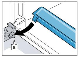
3. Slide the intermediate pane into the left- and right-hand retainers a.
