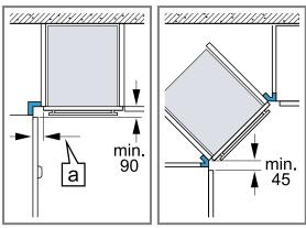
To ensure that the appliance door can be opened. vou must take the minimum dimensions into consideration when installing in a corner. The dimension a is dependent on the thickness of the unit front and the handle.
