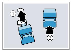
3. Hook the rear retainers with the hook into the top hole 1 and push them into the bottom hole 2.
