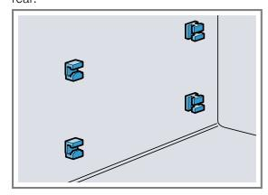
1. Hook the front retainers with the hook into the round hole at the top and set them at a slight angle ①.
