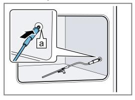
**5.** Place the small tube at the end of the connection hose into the container. If required, secure the small tube onto the container using the clip a.
