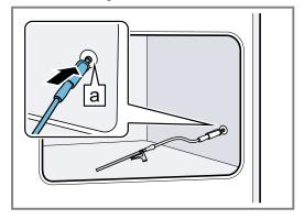
**6.** Position the small tube at the end of the connecting hose in the container so that all the liquid can be pumped into the appliance. If required, secure the small tube onto the container using the clip a.
