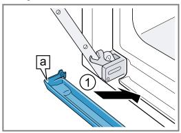
2. Snap the hooks a on the left and right of the condensate tray into the gap 1.
