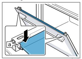
5. Note: When sliding the pane in, ensure that the glossy side of the pane is on the outside and the cut-outs on the left and right are at the top.
