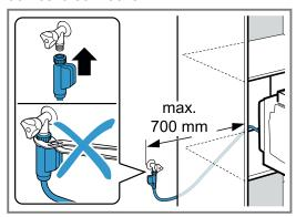
Only tighten the plastic union nut by hand. Do not subject the supply hose to tension, trap or squash it, or bend it too tightly.
