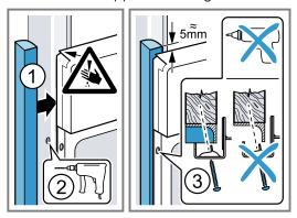
**Note:** The gap between the worktop and the appliance must not be closed by additional battens.
