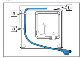
5. Install the supply hose with connection elbow on the domestic connection.
