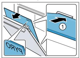
**5.** Push the inner pane in at the top ①. Push the sliding caps a downwards in the direction of the arrow.
