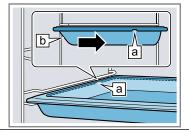
3. Push the accessory all the way in, making sure that it does not touch the appliance door.
