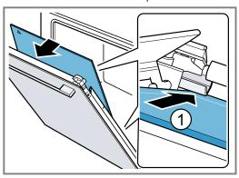
2. Note: The intermediate pane is automatically positioned by the rotational movement of the spacer.
