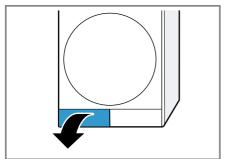
If you place a cloth beneath the maintenance flap, you can collect the remaining water from the base unit.
