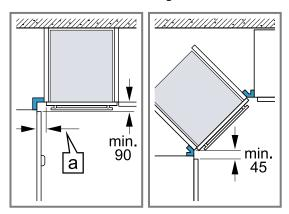
To ensure that the appliance door can be opened, you must take the minimum dimensions into consideration when installing in a corner. The dimension a is dependent on the thickness of the unit front and the handle.
