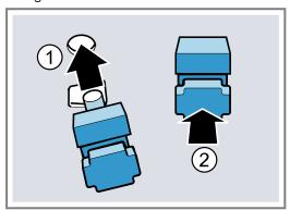
Hook the rear retainers with the hook into the top hole 1 and push them into the bottom hole 2.
