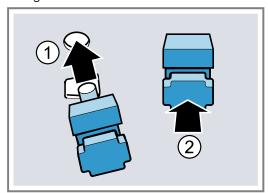
Hook the rear retainers with the hook into the top hole 1 and push them into the bottom hole 2.
