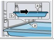
3. To place the accessory at shelf positions with pullout rails, pull out the pull-out rails.
