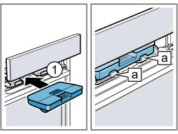
7. Slowly slide the control panel downwards and then push it away from you until it is closed completely.
