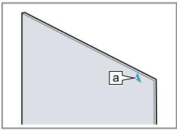
2. Insert the intermediate pane into the retainer a at the bottom ① and push it in firmly at the top.
