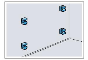
1. Hook the front retainers with the hook into the round hole at the top and set them at a slight angle ①.
