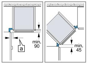
To ensure that the appliance door can be opened, you must take the minimum dimensions into consideration when installing in a corner. The dimension a is dependent on the thickness of the unit front and the handle.
