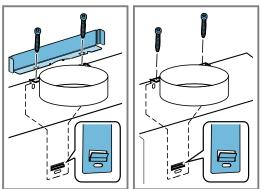
When you install a flue cover, install the bracket and hold it in place while screwing it in tight.
