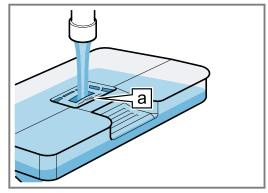
6. Slide the full water tank back into the recess ①. When doing so, make sure that the water tank clicks into place in the retainers a.
