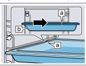
**3.** To place the accessory at shelf positions with pullout rails, pull out the pull-out rails.
