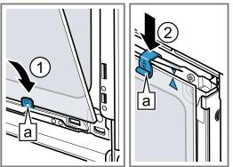
**4.** Attach the front pane downwards into the left- and right-hand retainers **a** ①.
