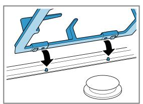
Place the cookware correctly on the pan supports. Never place the cookware directly on the burner. Always carefully remove the pan supports. When moving a pan support, the pan supports next to it may also move. **Tip:** You can remove the metal residue that remains when some items of cookware are moved on the pan support by cleaning it properly.
