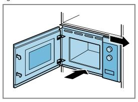
**4.** Screw the appliance in until the appliance is centrally aligned.
