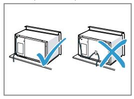
Insert the appliance into the unit and move it to the right.
