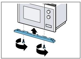
6. Secure the four supporting feet to the base of the microwave.
