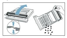
8. Rinse the fluff collector's filter thoroughly under running water and dry it.
