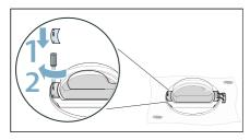
**Note:** Ensure that the door's seal is not jammed or damaged when inserting the eyelet.
