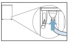
6. Secure the other side of the drain hose using the remaining accessories, depending on the connection situation.
