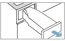
Turn the condensation container 180° onto its underside and remove the stopper that is fitted.
