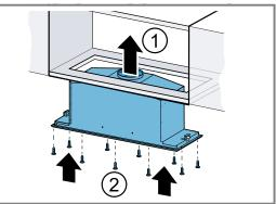
2. Tighten the fastening screws.
