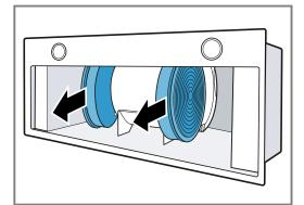
**3.** Guide the odour filter around the motor.
