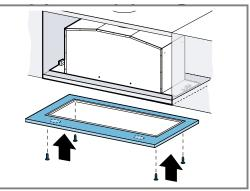
4. Secure the frame and the appliance with screws.
