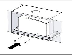
If the screws are not accessible from the exterior, the screws can also be fitted from the interior.
