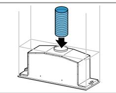
Establish the connection to the exhaust air opening.
