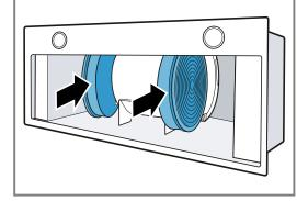
4. Install the grease filters.
