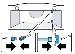
The plug can only be inserted into one position. 6. Ensure that the connector has engaged correctly.
