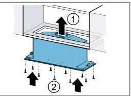
2. Tighten the fastening screws.
