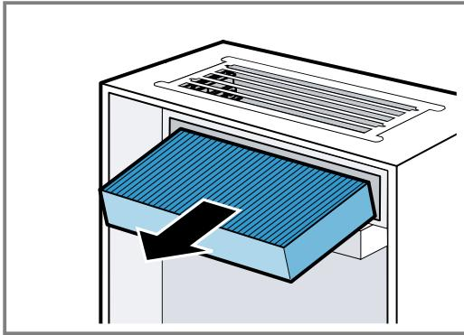
**Installing the odour filter for the CleanAir circulating-air module**
