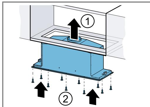
**2.** Tighten the fastening screws.
