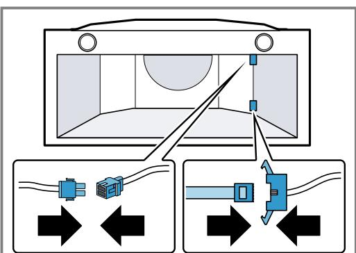
The plug can only be inserted into one position.
