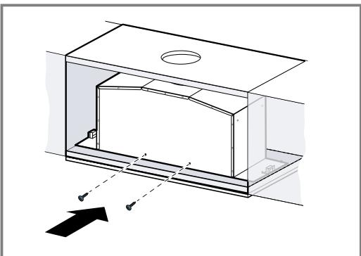
If the screws are not accessible from the exterior, the screws can also be fitted from the interior.
