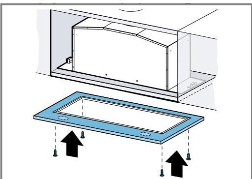
**4.** Secure the frame and the appliance with screws.
