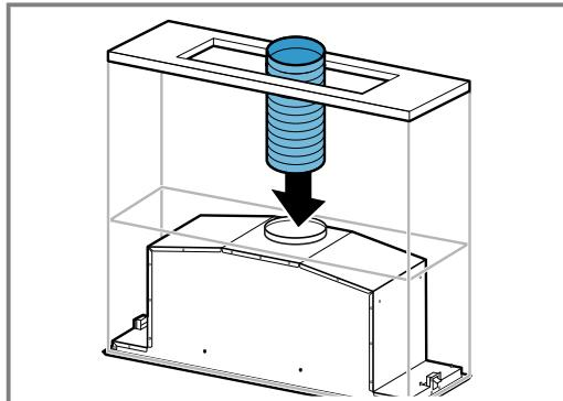
**2.** Establish the connection to the exhaust air opening.
