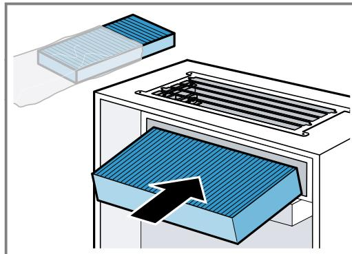
2. Insert the new odour filter into the circulating-air module.
