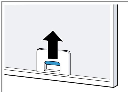
3. Remove the grease filters from the holders.
