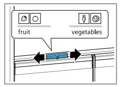
The air humidity in the fruit and vegetable container can be set according to the type and amount of food to be stored by moving the humidity control:
