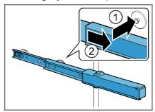
2. Place the telescopic rail on the rear pin ① and push the locking mechanism back 2.
